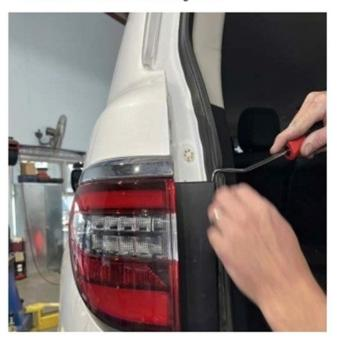
To remove the taillight you will need to push the rear of the light outwards to pop the clip on the side of the taillight
