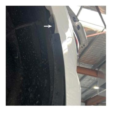
Take cover off side of taillight and remove the bolts behind it that hold the taillight on.
