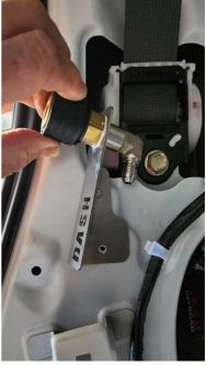
8. You will need to modify lower plastic quarter trim by drilling out x5 plastic welds and remove inside plastic Housing. Take care not to drill too deep
