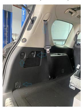
3. Place stencil on upper plastic trim and mark centre for outlet hole. Drill hole using a 51mm hole saw. Clean up hole and fit supplied rubber grommet.
