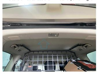
2. Remove floor panels and left upper and lower plastic trims. Use care as they can crack easily.
