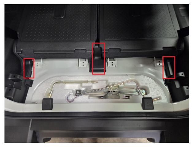
3. Remove the 4 14mm bolts holding the seats down.
