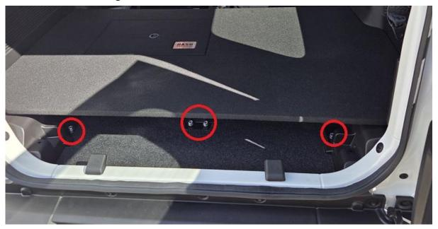
11. Fit the bolts and flange nuts to the front support brackets as shown. Hold the nuts under the bracket and screw in the bolts and washers on both sides.
