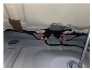
5. Remove the centre bracket trim to access the bolts and remove the 4 14mm bolts holding the seats down. Remove the 2 14mm nuts attaching the seatbelts to the side brackets. Unplug the seatbelt sensor connectors.
