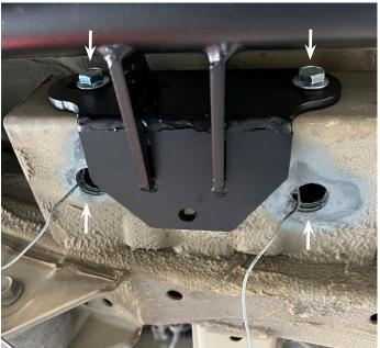
5. Drill the centre hole on the rear mount through the bottom and top of the box section and bolt with M10x110mm, flange nut and 50mm washer on top.
