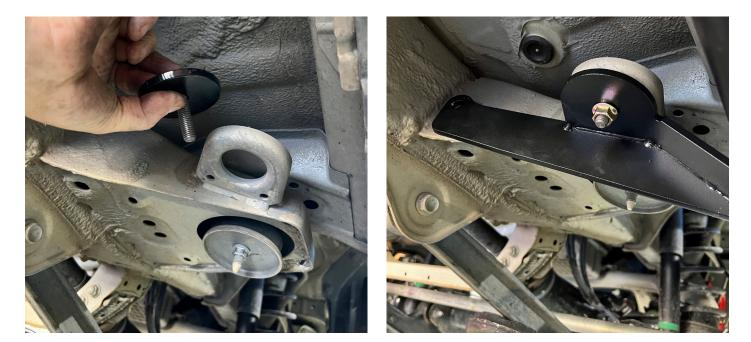
2. Drill out the 2 outer holes on the rear mount to 22mm to allow access for the flange nuts on wire
