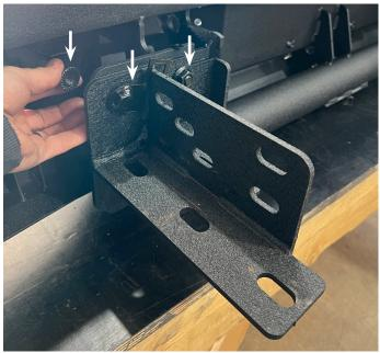
5. Fit the bar to the chassis with the existing tow bar bolts or M12x40mm bolts supplied. 3 bolts to the base of the chassis and 2 bolts to the inside, leave finger tight for now.
