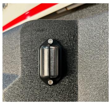
9. Remove the numberplate light loom/plug from the old bumper and wire to the new lights and connect plug back onto the ute loom.
