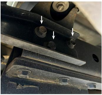
3. Unbolt and remove existing tow bar if fitted - 6 bolts each side
