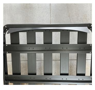
12. Bolt the wind deflector onto place. The access is tight so use the supplied allen key.
