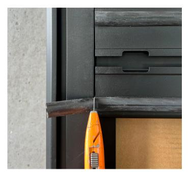
14. Before you install the roof rails you will need to remove the plastic cover from the trim on you patrol.
