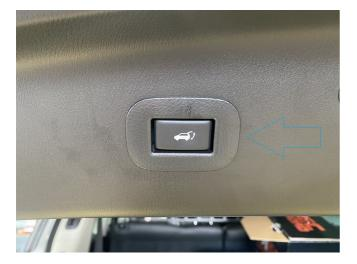
15. Use the provided template to mark the LH upper tailgate trim, cut out the oval hole and use the provided rubber strip to finish it off.
