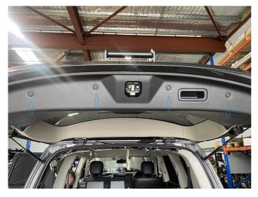
3. Remove the screw in the ceiling trim.
