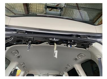
2. Remove the ceiling trim, being careful not to lose the metal clips from the light.
