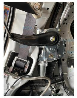
8. Connect the ground/Eearth wire to the original car D-pillar main ground line.
