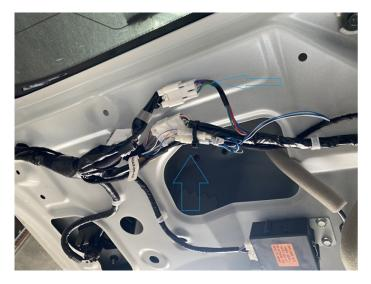
13. Plug in the Patch Loom for the tailgate harness.
