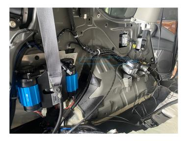
9. Remove the B-pillar trim panel, and connect the green central control unlocking.
