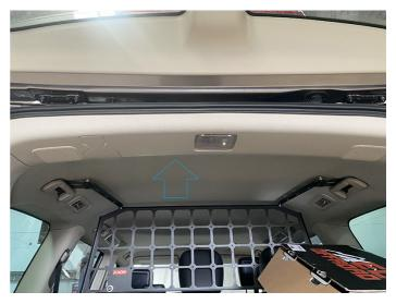
5. Remove the upper trim and feed the seatbelt back through the hole so you can get it right out of the way
