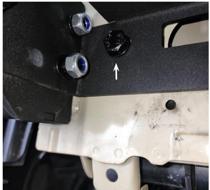
7. Insert the backing plate with 2x M10x70mm bolts and crush tubes in front of the radiator and through to the winch cradle and fit nuts and washers
