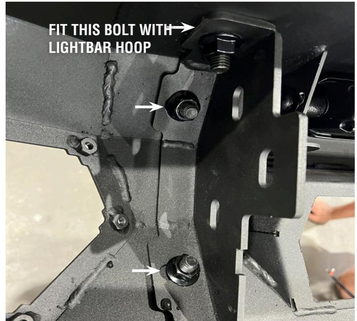
10. At the same time as fitting the brackets fit lightbar inside hoop and bolt the hoop to the bar with the two top bracket bolts
