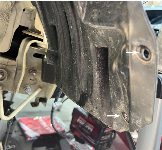
3. Remove the 3 bolts along the bottom of the bumper and remove bumper from the car
