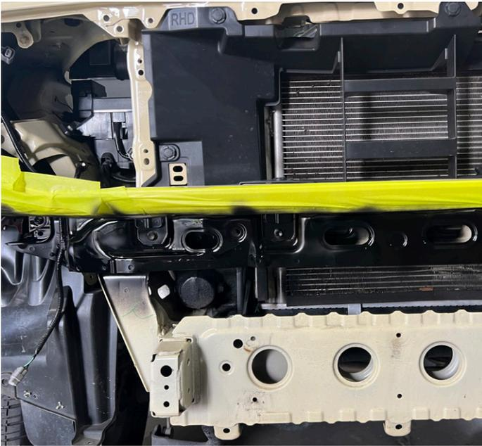
9. Fit the brackets to the bullbar with M12x30mm Button head bolts, measure the width of the cradle mounts and ensure bar mounts match so the bar can slide straight on.
