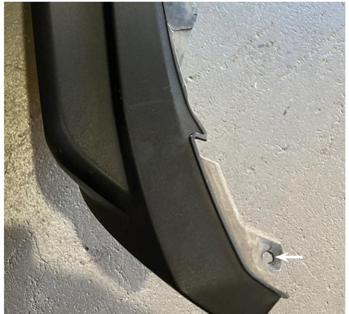
2. Remove the 2 clips on the inner guard
