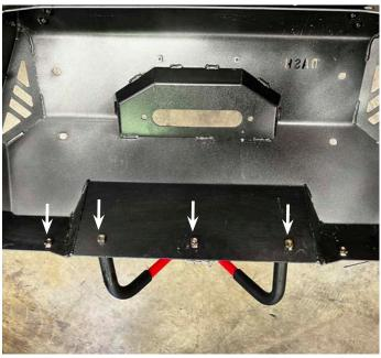
25. Mount the bar with 6x M10 Button head bolts with washers, 4 bolts in the front and 2 in top.
