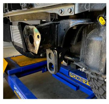
14. Attach the winch cradle with the 4 Factory bolts to the front of the chassis
