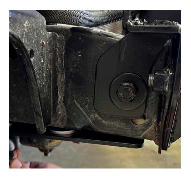
16. Fit the chassis support brackets to the chassis where the recovery points are mounted. Use the bolts in the recovery brackets bag. (See Below) If recovery points are being fitted, attach these now.
