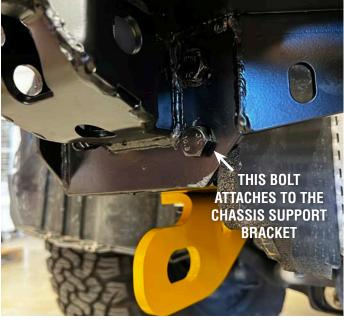
19. Fit the bumper brackets with M12x30mm Bolts and flange nuts. Make sure the bracket is pulled as far forward as possible and the nuts are on the outside making it easier to loosen if adjustment is need later.
