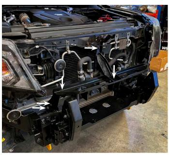
22. Bolt the bar wings to the centre or bar with M10x20mm bolts and flange nuts.
