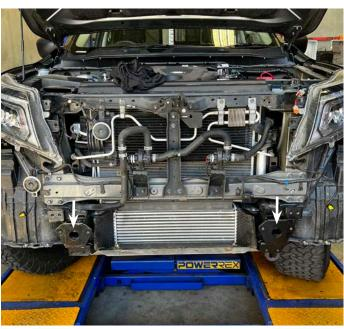
9. Remove the horn below the drivers headlight, this will be relocated later.
