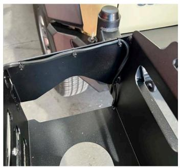
21. Fit and wire reverse lights - If you want to wire in 2 lights an additional relay is required for the second light (Relay not included in kit)
