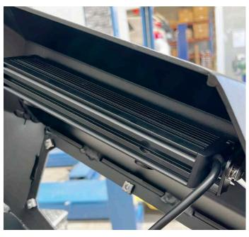
20. Fit the bar with 4x M10x30mm Button bolts and washers. Finger tight first, align bar and then tighten. Be careful when tightening that the washer doesn't damage the paint on the bar.
