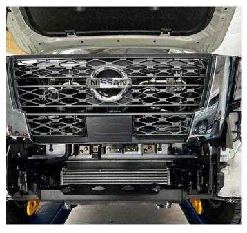
15. Fit bumper support brackets with 3x M12botls with washers and Nylon lock nuts, Leave finger tight. Place centre panel into position on bumper support panels, adjust alignment and tighten bumper support panel bolts.
