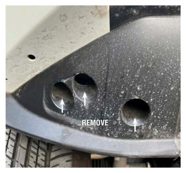
2. Remove the screw on the front of the inner guard. Once this is done carefully flex the inner guard t access and remove the bolt attaching the bumper to the outer guard
