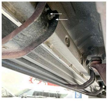
3. Mount the brackets to the steps with the M10x30mm Button Head Bolts/washers Flange Nuts. The rear and centre brackets are the same length the rear has 2 mounting holes where the centre has one mounting hole. and the longer bracket goes on the front.
