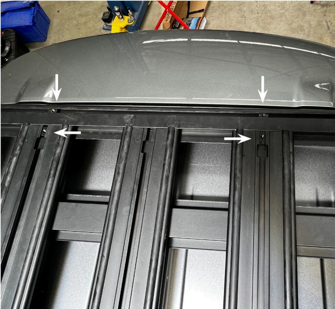
3. Use the 4 x M8 Button head bolts and bolt the top of the ladder in place.
