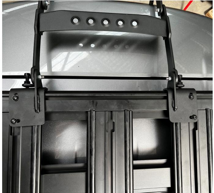
4. Adjust the bolt below to raise the rack so that it clears the spoiler and the base plate aligns with the existing number plate holes.
