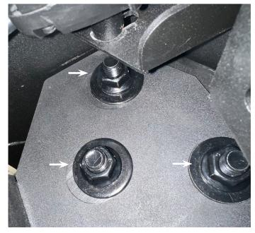
12. Mount wing support brackets with M10x20mm Bolts
