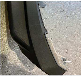
2. Remove the 2 clips on the inner guard
