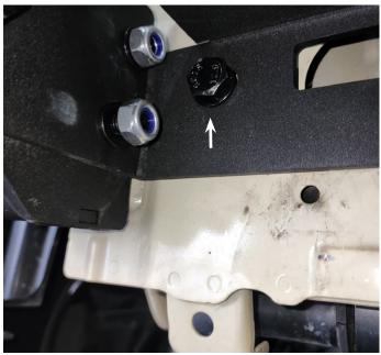
7. Insert the backing plate with 2x M10x70mm bolts and crush tubes in front of the radiator and through to the winch cradle and fit nuts and washers If winch is also being installed, fit this now.
