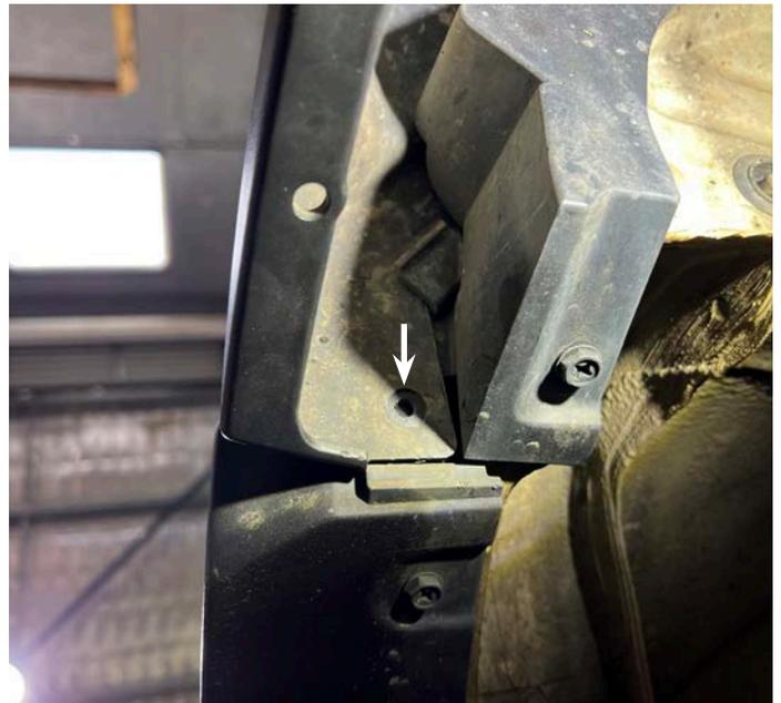
3. Remove 2 bolts that bolt to the chassis rails
