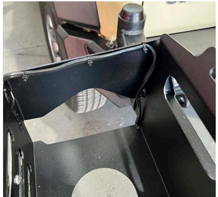
21. Fit and wire reverse lights - If you want to wire in 2 lights an additional relay is required for the second light (Relay not included in kit)
