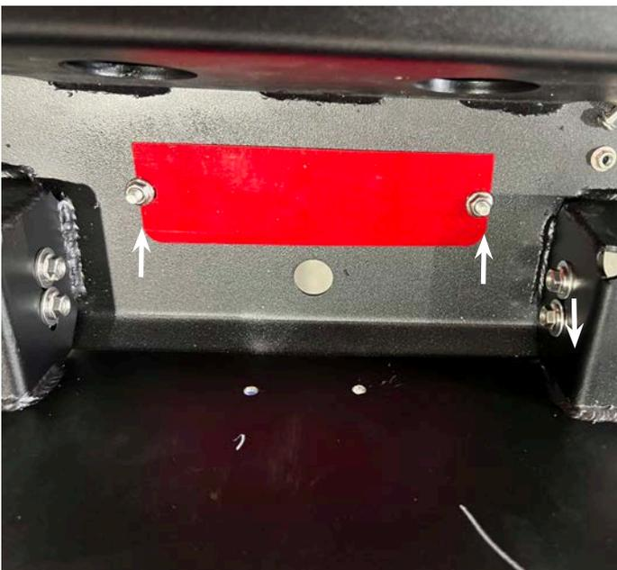
12. Fit the reverse camera to the bracket on the rear bar
