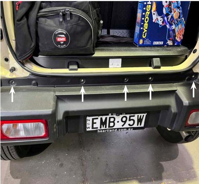
2. Remove the bolt that bolts the bumper to the wheel flare
