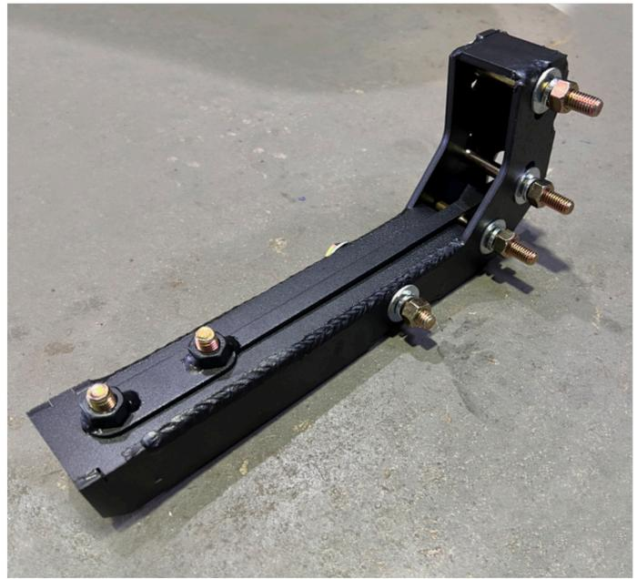
7. Slide the bracket in and bolt through the chassis with M10x70mm Full threaded bolts with washers and lock washer
