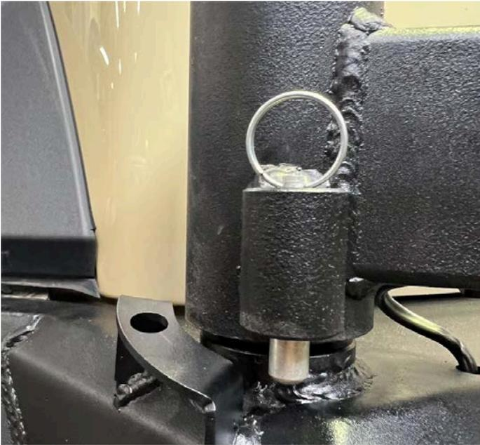
17. Fit swingaway latches, test and adjust latch and receiver until arms close firmly
