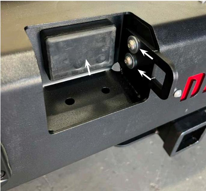
14. Mount the bar to the Jimny with 6 x M10x80mm Bolts with washers and lock washers
