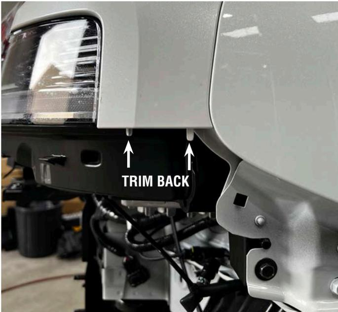
16. Mask up and paint the edge under the front of the guard black to create a shadow line
