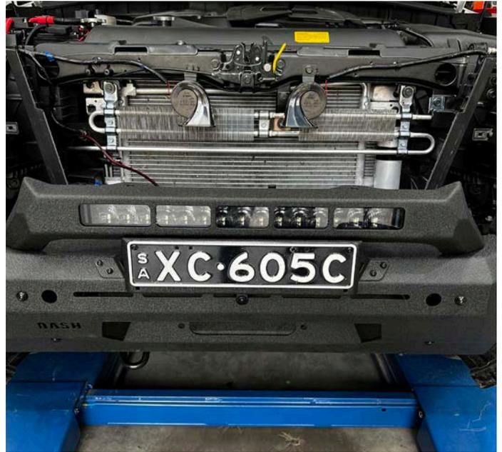
28. Mount the wing support brackets with 5x M10 flange nuts. tighten the nuts on the centre support first, adjust the wing to align with the guard, there should be approx a 20mm gap, then once correct tighten the wing nuts.
