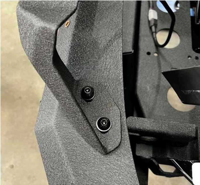
27. Mount the numberplate bracket with 4x M6 Button head bolts and washers
