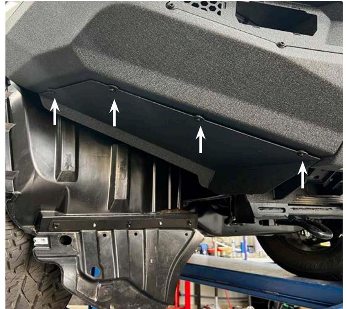
38. Fit the centre lower panels with M8 Button head bolts and washers
