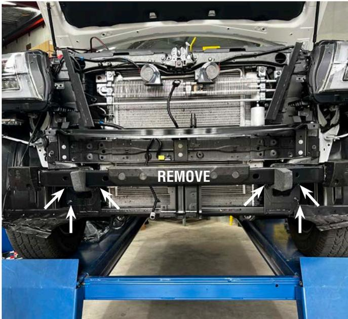
14. Cut the grille support panel as marked below and unbolt the centre
