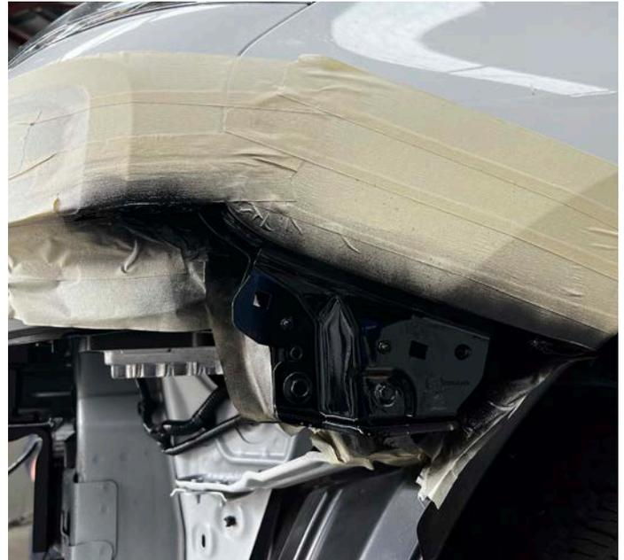
17. To relocate the radar you will need to have purchased the radar relocation bracket available on the Dash Offroad website. This mounts into the lower brace in front of the radiator. You will need to insert captive nuts into the 2 existing holes, or drill the holes through and use bolts (Rivet nuts and bolts for this are not included in the kit)
