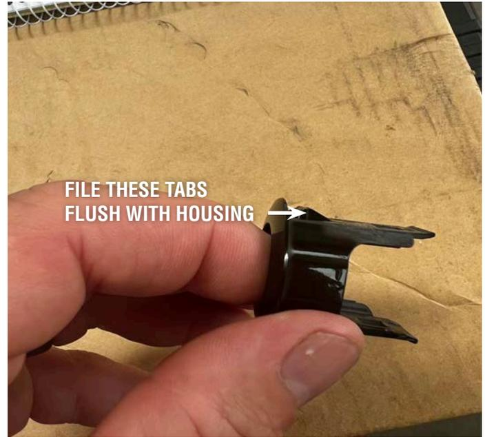
35. Fit the sensor mounts, wiring loom and sensors. You will need to cable tie the loom along the bracket below the radiator
