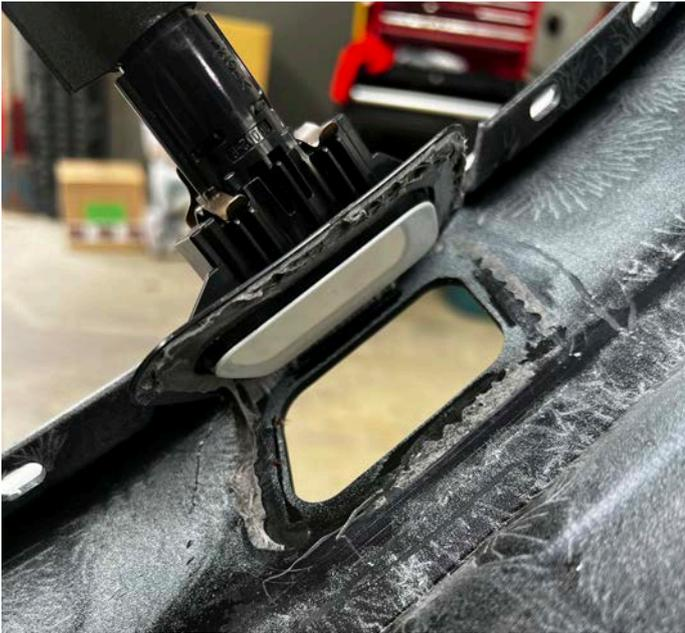
31. The headlight washers mount on the opposite sides to where they came out of the bumper so you will need to rotate the washer heads 90 degree
