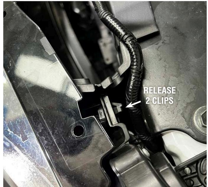
3. Release the base grille clips and unplug the camera
