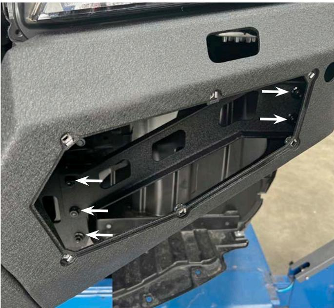
29. Once the bullbar is all aligned and tightened fit 4x M8 Bolts with flange nuts to the locating pins where the bar supports mount to the centre winch cradle.
