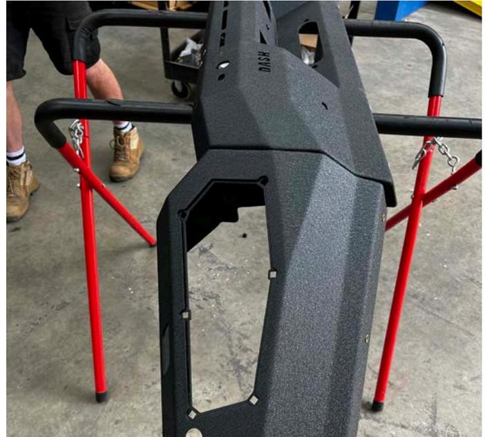
22. Remove the factory camera from the grille and remove the plug clip from the bracket. Bend the bracket and to align the camera with the hole in the bar and drill and bolt through the bottom of the bar with a M8 bolt and nut.
