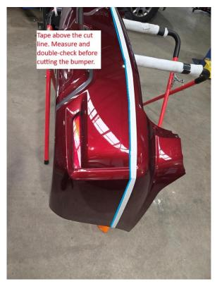
17. Confirm you have allowed 10-20 mm extra for the first cut. This will allow the bumper to be fitted and marked in place. Cut the bumper along the marked line with an air hacksaw or similar.
