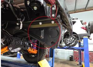
6. Remove the Blind spot radars and all of the mounting brackets. Be careful with the radars and keep them separate to refit on the same sides.
