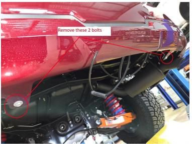
4. Apply masking tape to the rear quarter panel as shown. Carefully pull out the front corner of the plastic bumper to dislodge the retaining clips. Pull the bumper away from the car and disconnect the park sensor loom connector on the right side of the bumper.
