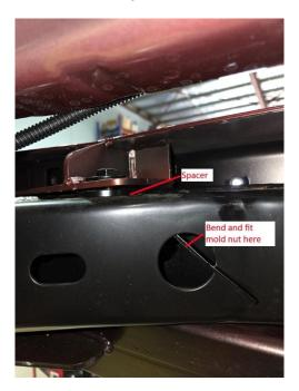
14. Tighten the 4 rear M12 bolts until they are firm only. Tighten the 6 x Chassis mounting bolts to 92nm, then tighten the 4 rear bolts to 92 nm also, tighten the 4 side M8 bolts as required. Tighten the 2 top mounting bolts.
