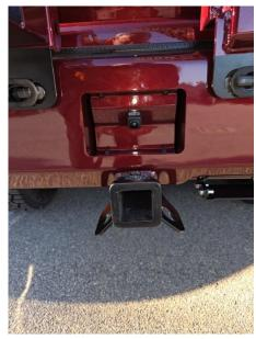
25. Run the wiring loom for the rear lights into the quarter panel through the grommet in the bottom of the left rear guard, with the inner plastic panel removed, connect to the factory trailer wiring plug, and connect the earth wire to the 10mm bolt nearby.
