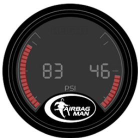
SUPPLIED MODE - BEZEL CELLS DISPLAY PRESSURE 0-100PSI
