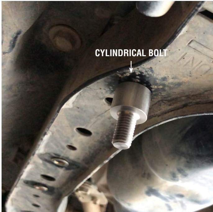
ONE OF FOUR CYLINDRICAL BOLTS INSERTED INTO BACK RAIL
