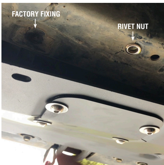
RIVET NUT INSERTED ON FRONT RAIL
