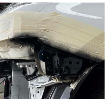
17. To relocate the radar you will need to have purchased the radar relocation bracket available on the Dash Offroad website. This mounts into the lower brace in front of the radiator. You will need to insert captive nuts into the 2 existing holes, or drill the holes through and use bolts (Rivet nuts and bolts for this are not included in the kit)
