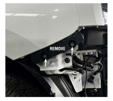
11. Unbolt the radar (TIL Models only) and move to side to relocate later. TI Models radar position does not need moving
