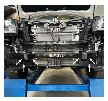
14. Cut the grille support panel as marked below and unbolt the centre
