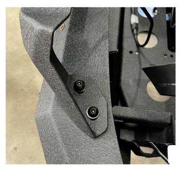
28. Mount the wing support brackets with 5x M10 flange nuts. tighten the nuts on the centre support first, adjust the wing to align with the guard, there should be approx a 20mm gap, then once correct tighen the wing nuts. 27. Mount the numberplate bracket with 4x M6 Button head bolts and washers
