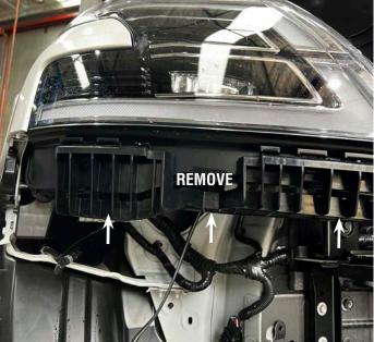
12. Remove the two air dam reflectors.
