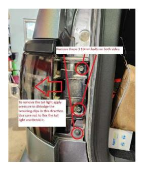
2. Pull the taillight loom and grommet out and disconnect the taillight. Remove the plastic clip on both sides.
