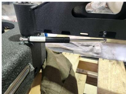
21. Attach the swing arm latch, adjust it, and tighten it as needed. Fit the spare wheel flange using the longest bolt, but don't tighten it. Fit the spare wheel to the arm. Push the wheel towards the vehicle fully, then tighten the head bolt. Fit the other bolts to the head and tighten.
