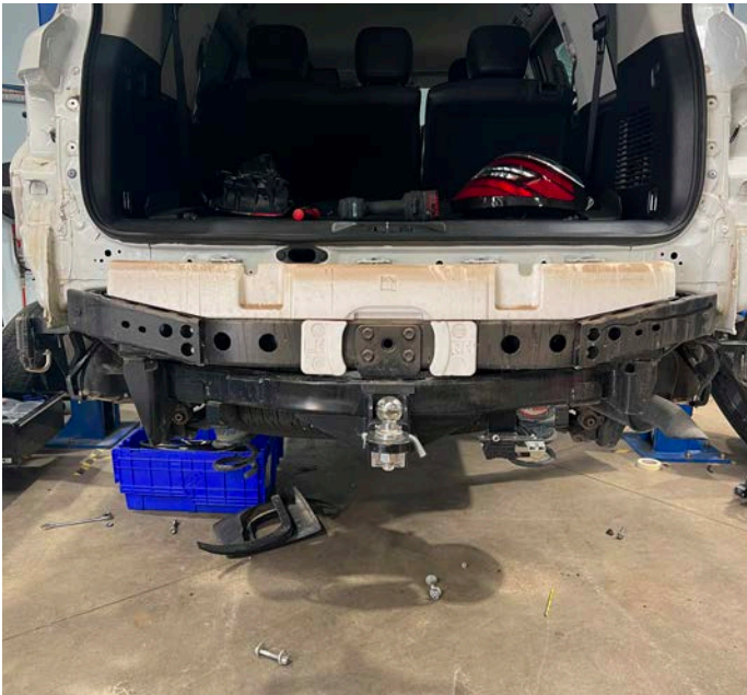
11. Remove the 4 bolts from the back of the towbar and remove towbar.
