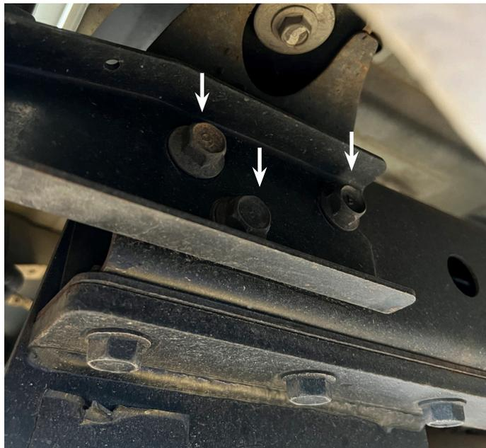
3. Unbolt and remove existing tow bar if fitted - 6 bolts each side
