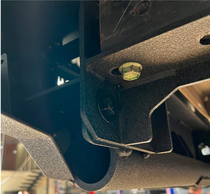
8. Fit the numberplate lights with M4 Hex bolts and nuts.
