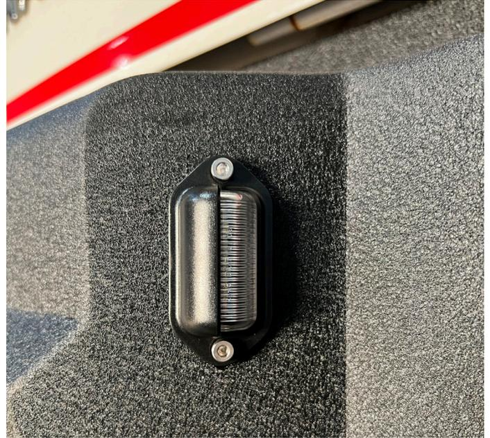
9. Remove the numberplate light loom/plug from the old bumper and wire to the new lights and connect plug back onto the ute loom.
