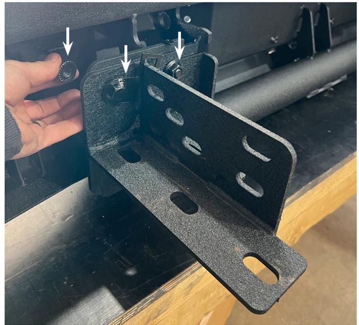
5. Fit the bar to the chassis with the existing tow bar bolts or M12x40mm bolts supplied. 3 bolts to the base of the chassis and 2 bolts to the inside, leave finger tight for now.
