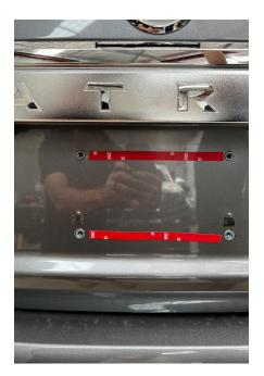
6. Remove the number plate bolts, lift the base plate out of the way and drill and insert the 2 M8 Nutserts (It is recommended to paint the holes before inserting the nutserts)
