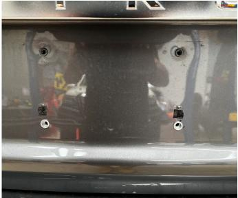
IF YOU DO NOT HAVE A RIVET GUN THESE CAN BE INSERTED MANUALLY - SEE 'DASH OFFROAD BASH PLATE INSTALL" ON YOU TUBE FOR MORE DETAILED INSTRUCTIONS ON THIS PROCESS
