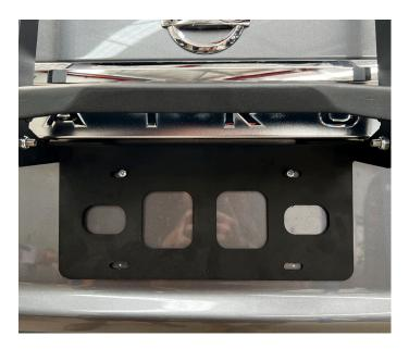
It is recommended to apply some sponge double sided tape or similar (Not supplied) to the tailgate before bolting up the base plate to avoid scratching the paint.
