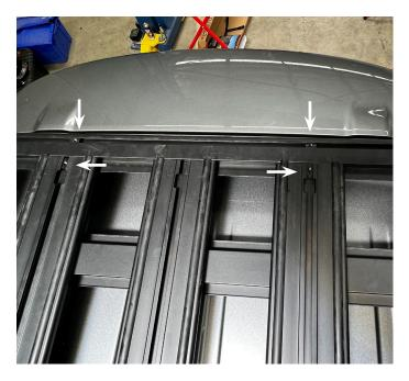
4. Adjust the bolt below to raise the rack so that it clears the spoiler and the base plate aligns with the existing number plate holes.
