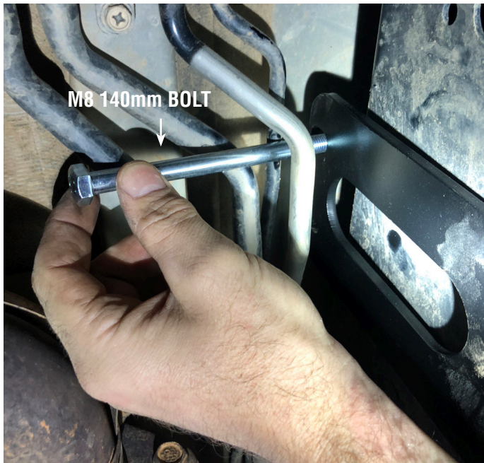
BOLT INSERTED INTO MIDDLE BRACKET
