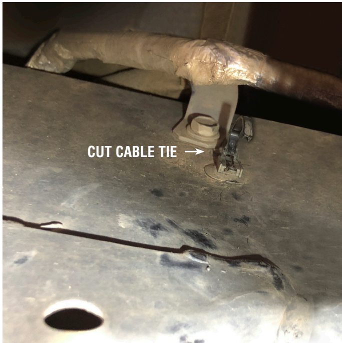
CHASSIS WHERE REAR BRACKET WILL MOUNT
