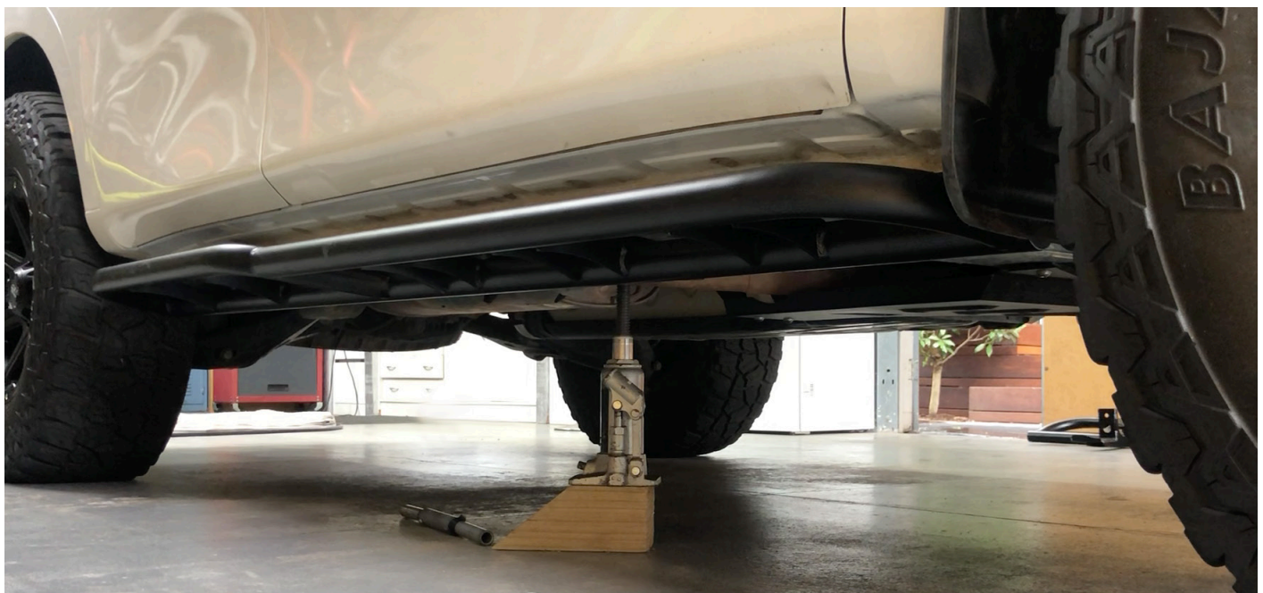
SLIDER HELD IN POSITION WITH JACK
