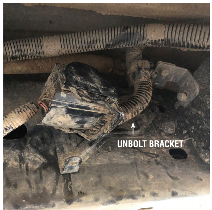
BRACKET AND PLUG UNDER PLASTIC COVER
