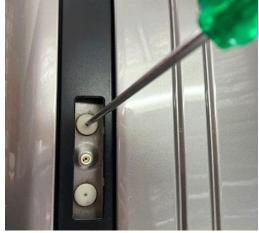
TIL Models you will need to remove the factory roof rails. The trim over the centre mounting point will need to be trimmed using a small pair of tin snips as shown. Mark and cut the Centre mounting trim towards the rear of the vehicle and extend the opening by 55mm. To expose the second mounting hole.
