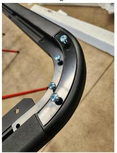
2. Fit M6 channel nuts and slide along to line up with holes in the inner corner supports and fit 8 M6 x 12mm hex head bolts to each corner but don't tighten yet. Place 5 long platform rails one at a time under frame and align holes in ends and fit M6 x 15mm hex head bolts loosely into each end.
