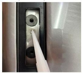
7. To bolt the roof rails down use the M8x25mm Stainless Steel Bolt with one 8x16mm washer. Apply some silicone to the thread of the bolt to ensure that the holes in the roof channel are waterproof when the bolt is in and tightened. Put the roof rails in place. Start with the bolts in the centre mount, then the front mount, and finally the back mount. Put all bolts in finger tight first before fully tightening.
