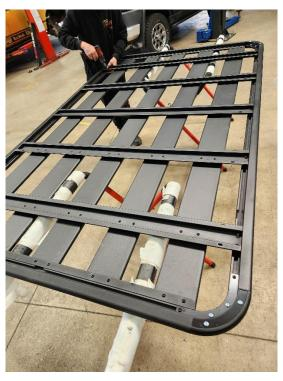
4. Attach wind deflector by inserting 4 x M6 channel nuts into front rail of roof rack (any end you like). Place the wind deflector and align the channel nuts as required. Fit 4 M6x12 hex bolts loosely. Centre wind deflector and tighten bolts.
