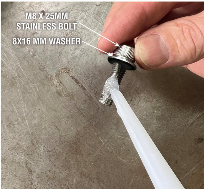
20. Put the roof rails in place. Start with the bolts in the centre mount, then the front mount, and finally the back mount. Put all bolts in finger tight first before fully tightening.
