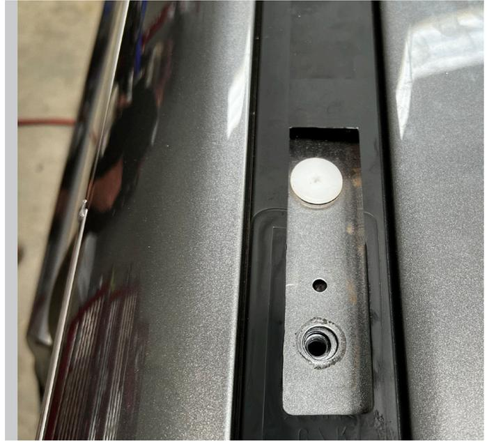
17. Place the 8x25mm rubber washers onto each of the bolt holes, you can also add silicone under these for additional sealing.
