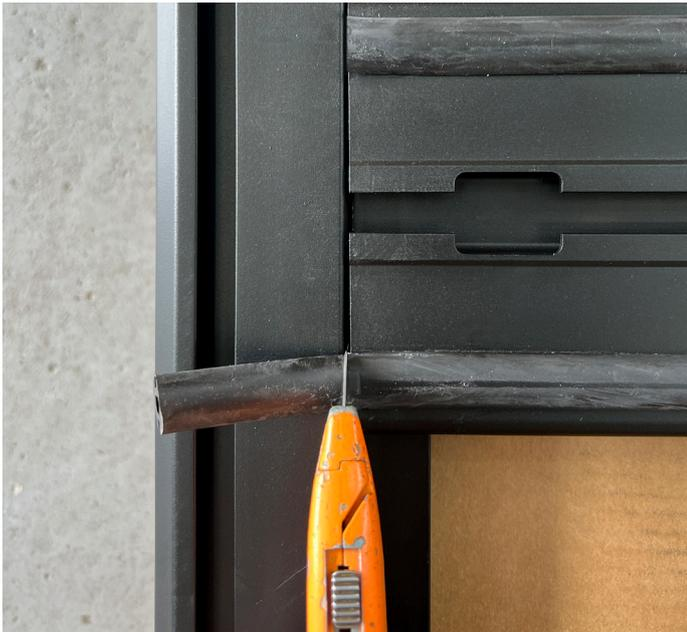
14. Before you install the roof rails you will need to remove the plastic cover from the trim on your patrol.
