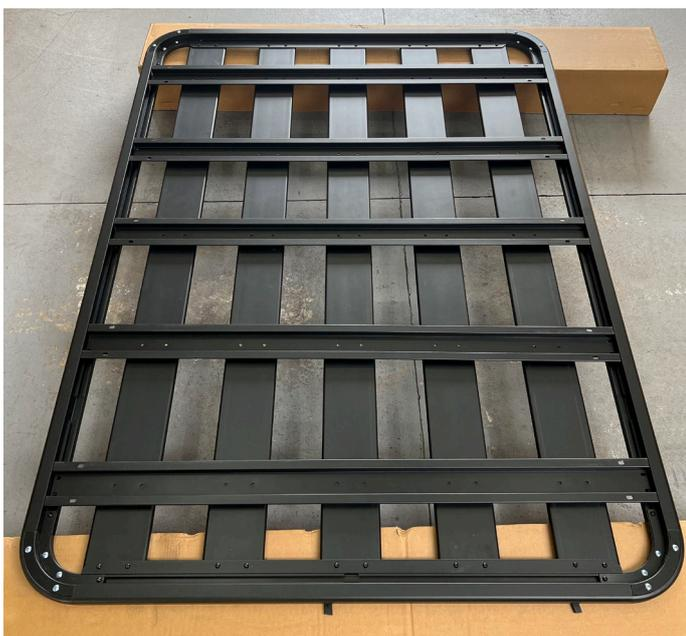
8. Bolt the 5 cross rails to the platform rails.
