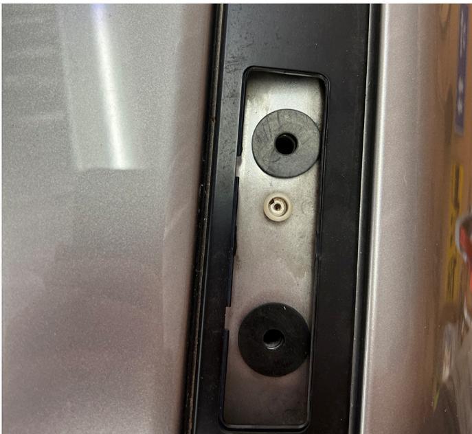
18. Add some silicone to the bolt holes and silicone inside the white cap to seal it up.
