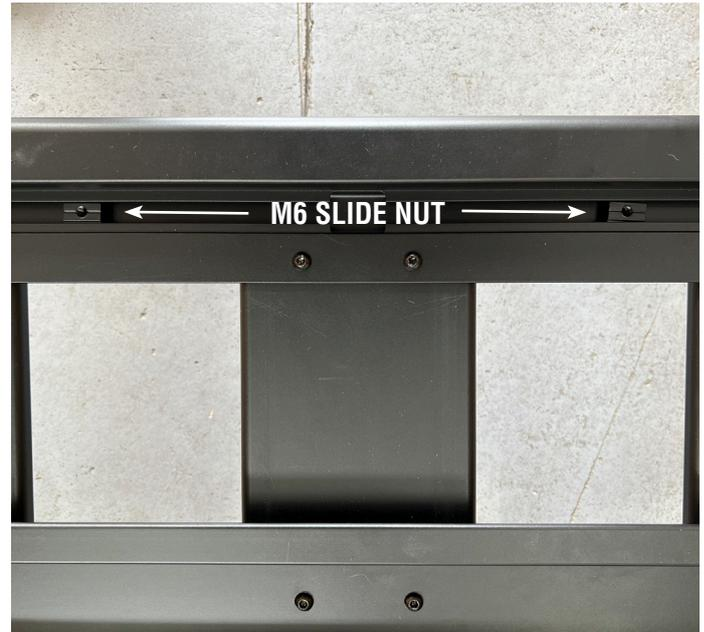
11. Place the wind deflector in place ensuring it is facing backwards and align the 4 nutserts with the holes in the wind deflector.
