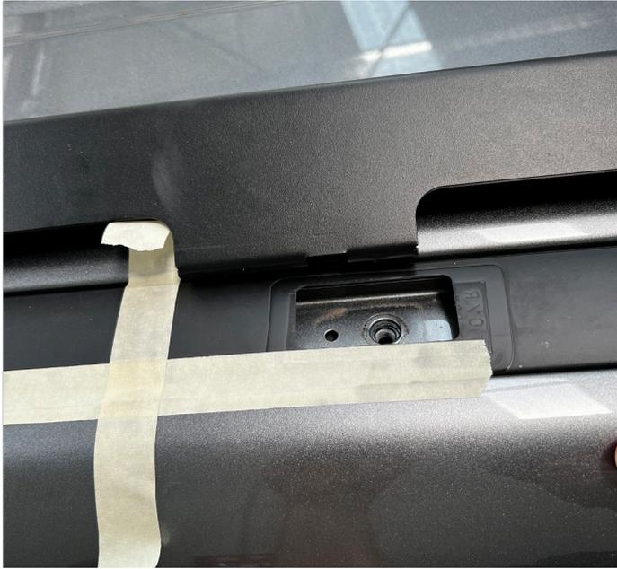
18. Cut with a small recircating saw or small grinder. This will expose a white cover over the second mounting hole, remove the cover.
