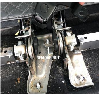
Please Note: If you are only using the left or right floor configuration and retaining one of the 3rd row seats then this seat does not need to unbolted.
